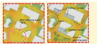
在戶外地方加設遮陽設計,如上蓋或樹蔭等,可帶來降溫效果。左圖為 加設遮陽設計前錄得較高的通用熱氣候指數的情況;右圖中綠色部分顯 示當加設遮陽設計後,相關指數下降,代表戶外舒適度有所改善。 In open spaces, shading devices, such as shelters or tree canopies, can bring improvement to thermal comfort. Photos on the left shows the scenario with relatively high universal thermal climate index (UTCI), whereas in photo on the right, after installing shading devices, there are improvements in the outdoor thermal comfort level as indicated by a lower UTCI index.
