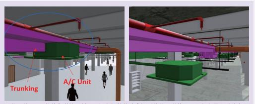
團隊可利用BIM軟件作碰撞分析,預視各設計範疇會遇到的位置碰撞問題。如左圖中以綠色顯示的空調設備,正好陷入了以紅色標示的管槽位置。右圖是解決碰撞問題後的改良設計。 With BIM software, clash analysis can be conducted to detect potential collision of elements in the design model. In the photo on the left, the air-conditioning unit (as shown in green) is colliding with the trunking (as shown in red). The photo on the right shows the rearrangement of the air-conditioning unit's position for solving the problem.
